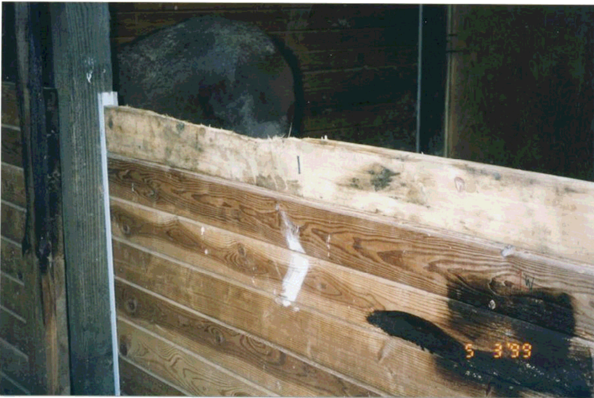
Top board in one of the ten stalls used in this experiment. The left end of the board is Douglas Fir while the right end is Western Juniper. Note the amount chewed from the Fir portion of the board compared to the Juniper.
