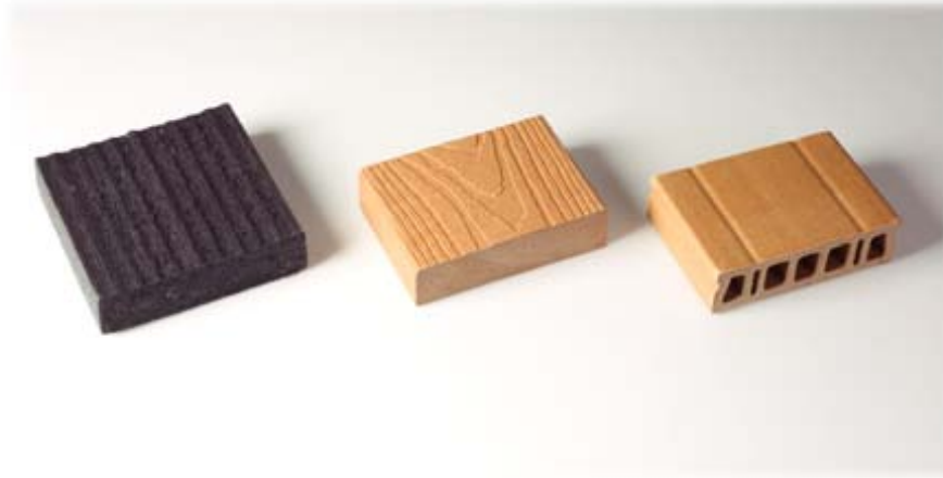
Figure 4—Alternatives to treated wood include rubber wood and solid- and hollow-core plastic-wood composite decking.
