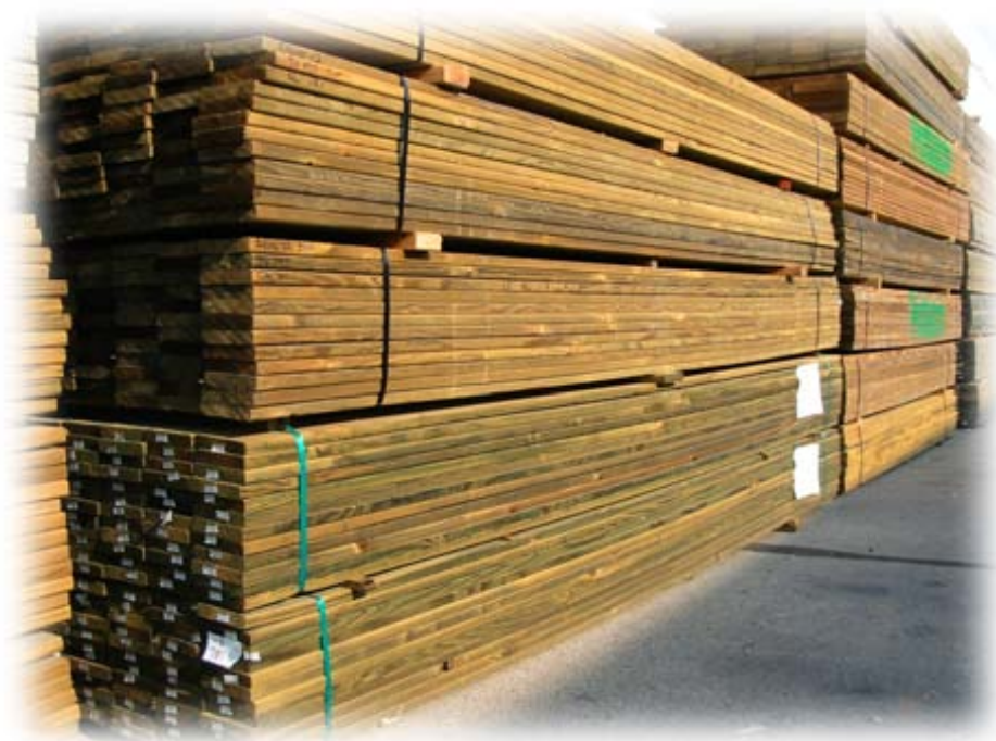
Figure 3—Pressure-treated lumber stockpiled at a lumberyard. Lumber treated with ACQ-D and CA-B has become widely available.
